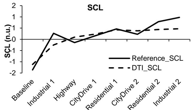
Figure 7: The average normalized skin conductance level per driving segment. The reference SCL is measured at the fingers. The DTI SCL is measured at the wrist.
