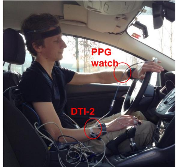
Figure 2 The sensors connected to a driver. The PPG watch to measure heart rate can be seen on the left wrist. The DTI-2 sensor bracelet to measure skin conductance can be seen at the right wrist. The small blue box is the NeXus device which is used for the wired reference measurements.
