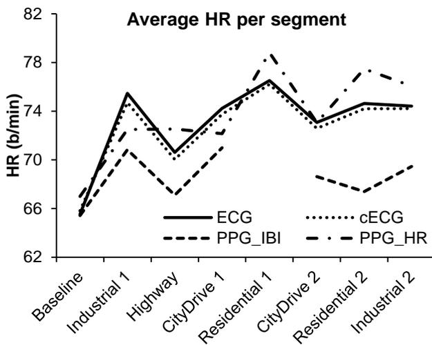
Figure 6: The average HR measured via the reference ECG, capacitive ECG (cECG), and the PPG. The PPG wrist signal has been analyzed in two ways, via exact successive detected IBI's (PPG\_IBI) and via the continuous averaged HR (PPG\_HR). No HR's were detected in the Residential 1 for PPG\_IBI, therefore a HR prediction is missing.
