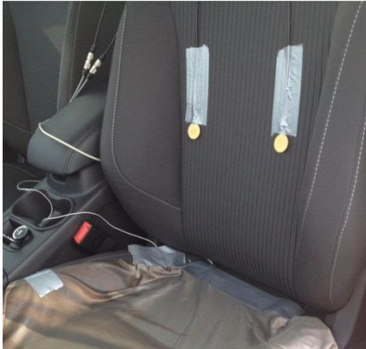
Figure 3 The two sensors of the capacitive ECG are connected to the back of the chair. The cloth acting as ground plate can be seen on the chair.
