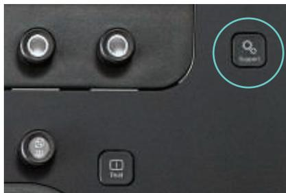
Support request button for immediate access to Philips support.
