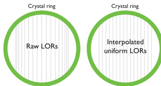
**Figure 8** Raw LORs (left) versus interpolated uniform LORs (right).
