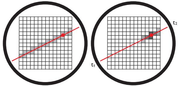
**Figure 7** In conventional PET (left) there is no localization along the line of response. Astonish TF technology (right) is able to pinpoint the annihilation event more precisely along the LOR.
