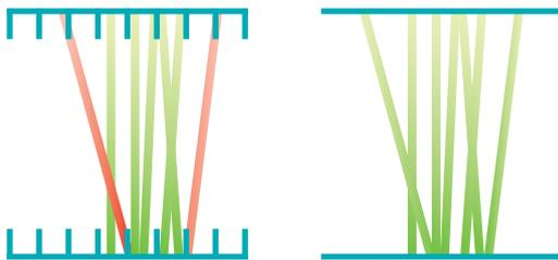
**Figure 6** In 2D mode (left) only 'in-plane' lines of response (LORs) are accepted. In 3D (right) LORs at all angles are accepted and the sensitivity is increased. 3D imaging leverages the advantages of fast, modern crystals with excellent light output and energy resolution.
