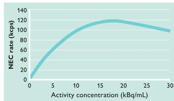
**Figure 5** NEC rate versus activity concentration for a NEMA countless cylindrical 20 cm diameter phantom.
