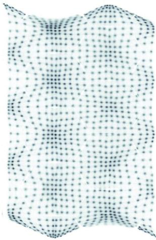
**Figure 3** Crystal map for one detector module. Each dark spot corresponds to an individual LYSO crystal. Good pixel separation is observed with Astonish TF technology, resolution, and reconstruction speed.
