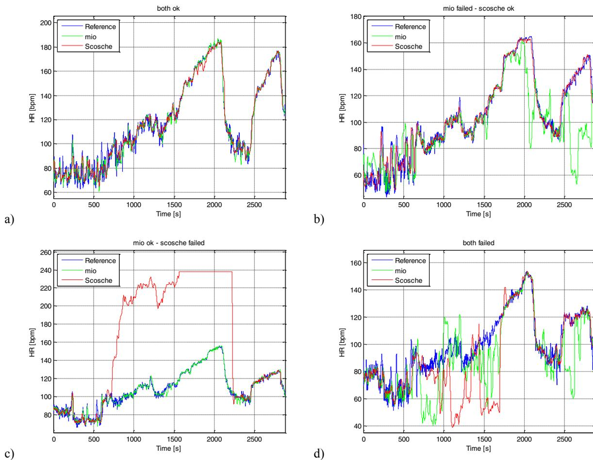
Figure 2. A) HR monitoring successful with both devices. B) Wrist based Mio Alpha fails during ergocycling. C) Forearm based Scosche Rhythm failed during walking and running, likely due to sensor displacement. D) Both devices show poor performance.
